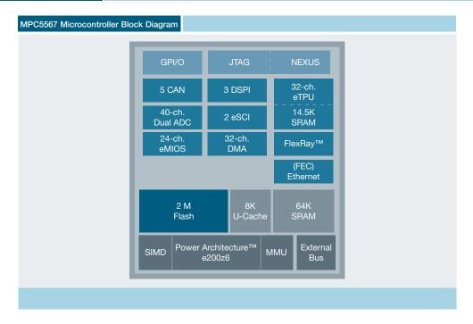
With the combined capabilities of FlexRay technology and Ethernet, along with five Controller Area Network (CAN) modules, the MPC5567 helps developers control costs when designing increasingly complex applications in automotive and industrial systems, such as:
